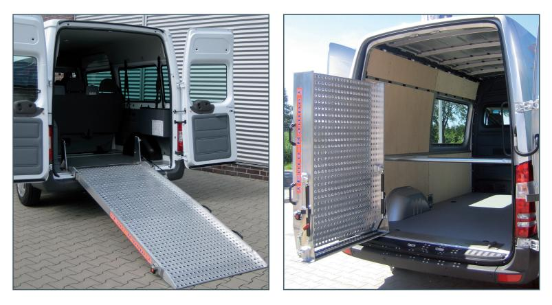
Wheelchair ramps for minivans or full-size vans make it easier to transport wheelchair passengers, speeding up entry and exiting considerably. SmartRamps are available in a range of lengths and widths. They are produced using perforated aluminum metal profiles that are lightweight, non-slip and ultra-strong. These ramps are available as straight fold-up or swivel-mounted.
